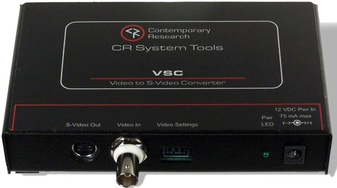
The VSC Video to S-Video Converter delivers high-quality S-Video signals from a composite video input. Employing technology developed for the popular 232-STS S-Video TV Tuner, the VSC features digital 2-D adaptive Y/C separation for superior S-Video performance. Front-panel settings allow video looping and selectively boost luminance (Y) and chrominance (C) video levels. NTSC and PAL versions available.
